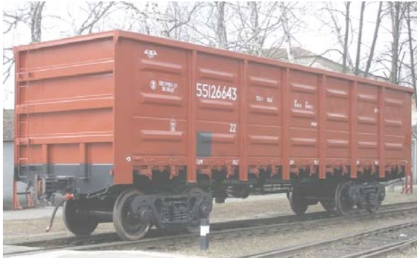
Fig. 5. Universal gondola car with unloading hatches in the floor of the model 12-7039
