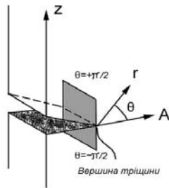
Fig. 1. The coordinates describing the dependence between the local deformations and stresses in the crack tip front
