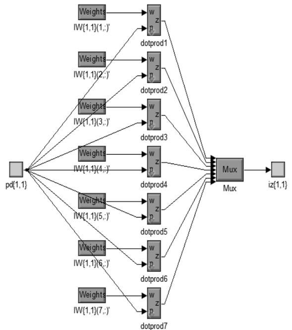
Fig.5. Model of the hidden layer of a neural network
