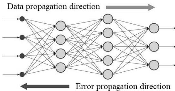
Fig.3. General scheme of neural network with back propagation of the error
