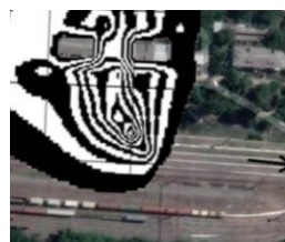
Figure 4. Predicted NO_2 concentration contours, level z = 3\text{m} , t = 15\text{s} .
