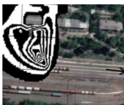
Figure 3. Predicted NO_2 concentration contours, level z = 3\text{m} , t = 8\text{s} .
