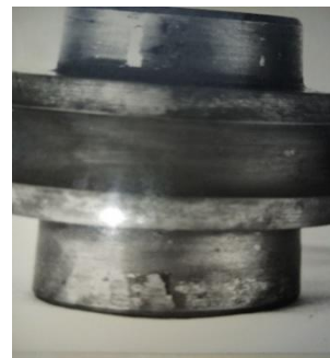
Fig. 5. Chipping of rollers
