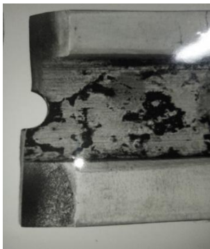
Fig. 2. Confessional wear on the working track of the support bar, developing to a depth of 0.2...0.4 mm
