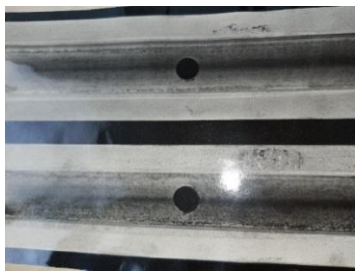
Fig. 3. The nature of the distribution of wear along the length of the working track of the bar
