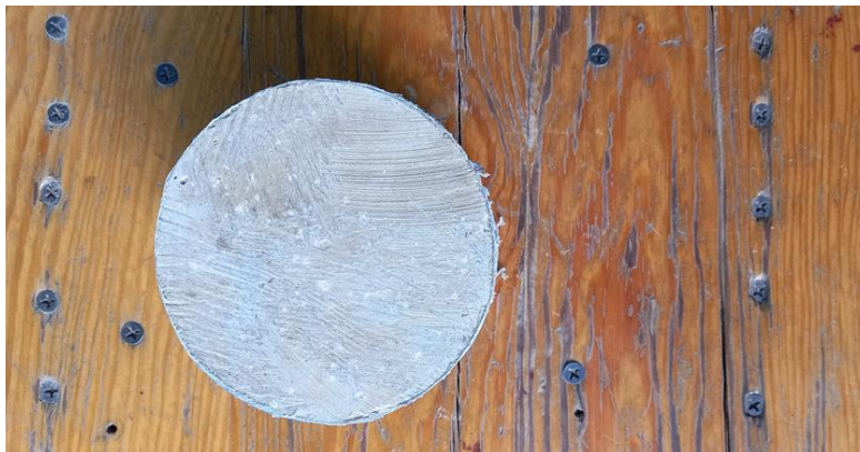
Figure 2. The view of the soil-cement sample after its processing.
