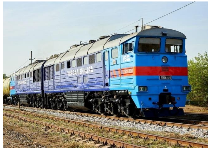
Figure 1. General appearance of the 2TE116 diesel locomotive (photo [30]). Non-English word means an element of the locomotive livery, which contains the name of the company in Ukrainian.
