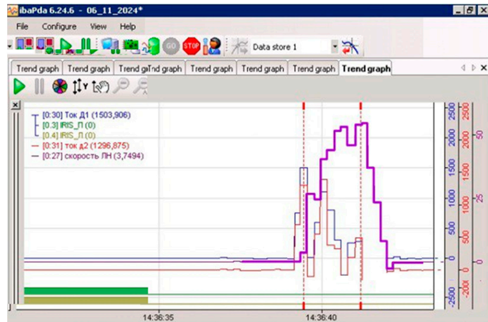
Figure 10. Registered transient process in the drum shears' mechanism.
