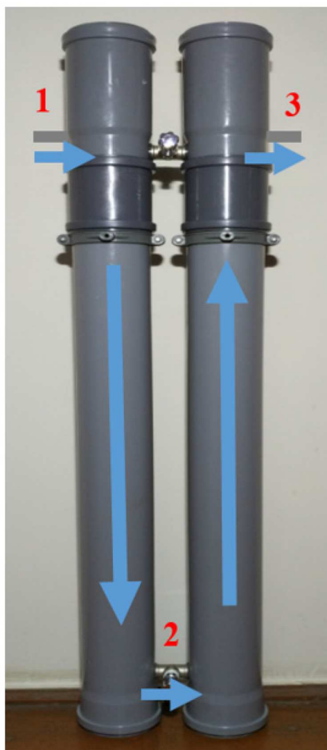
Figure 1. Photo of a biofilter and the trajectory of water shifts in it. '1', '2', '3' – points of sampling.
