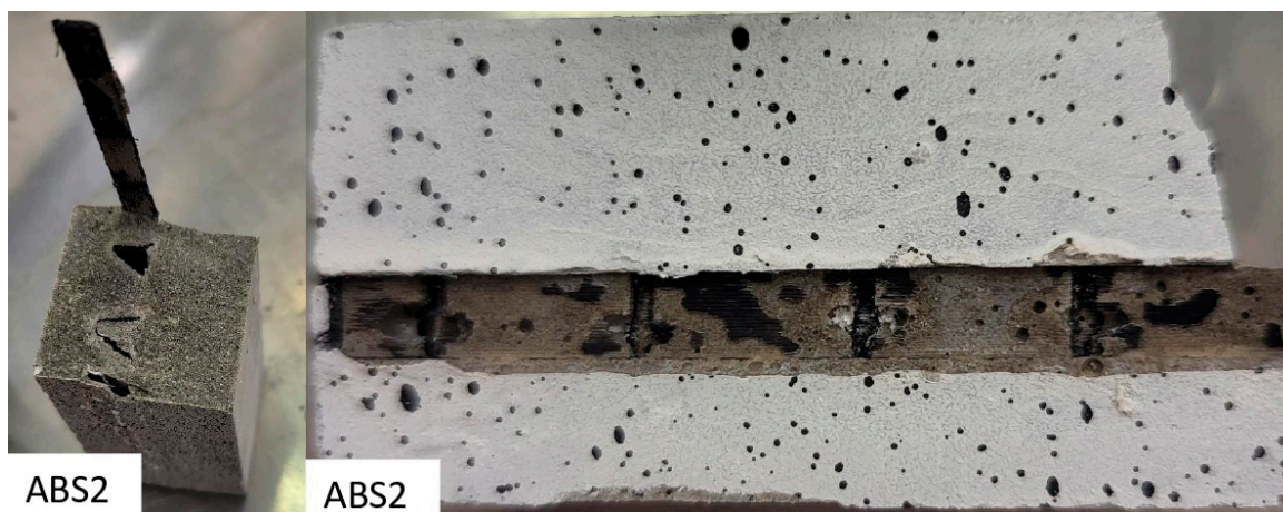
Figure 11. Separation of the ABS reinforcement from the concrete without adhering to white precipitation.
