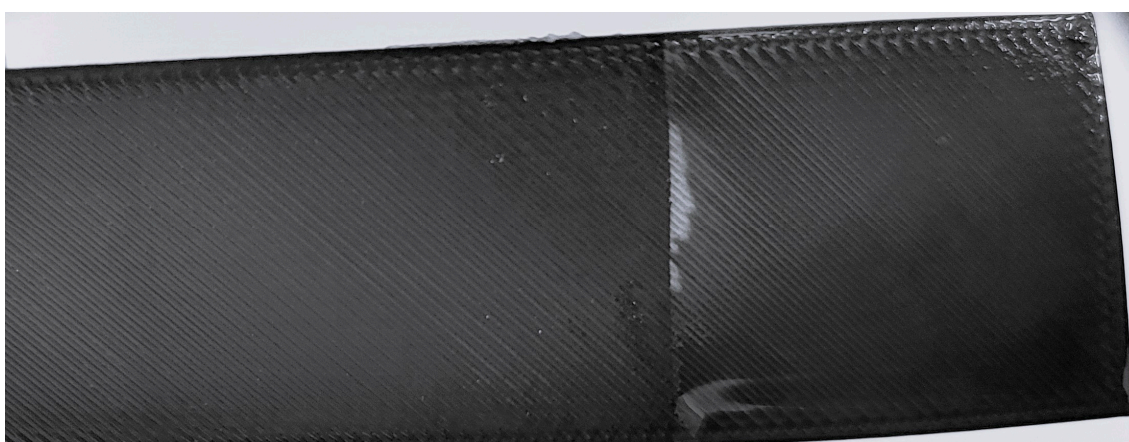
Figure 14. Fading of the color of the HI specimen immersed into the 12.55 pH solution with a small amount of white precipitation on day 7.
