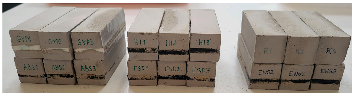
Figure 12. Surface of concrete specimens before DIC measurements (executed by GOM ATOS and GOM ARAMIS instruments).
