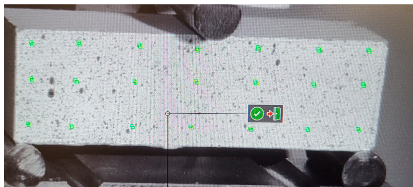
Figure 5. Experimental set-up with an appropriately painted surface, recognizable for the system.
