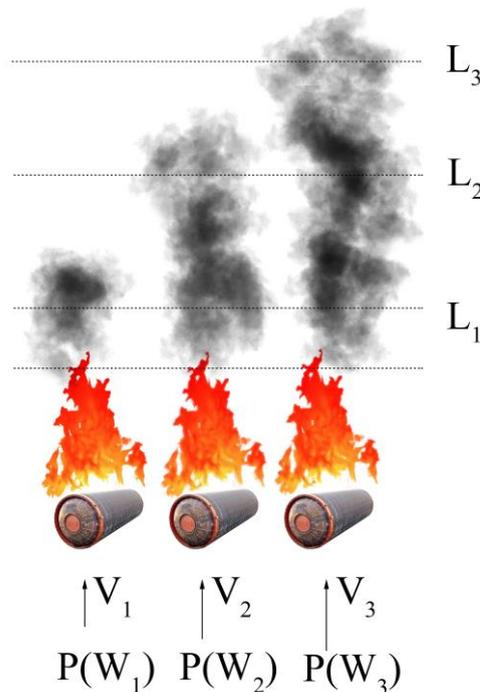
**Fig. 2.** Formation of hitting zone under different wind velocities [15]
