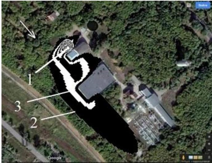
**Fig. 4.** Contamination zone ( $Cl_2$ ),  $t=21s$ : 1 – emission place; 2 – concentration  $C= 250\text{ mg/m}^3$ ; 3 – concentration  $C=1250\text{ mg/m}^3$
