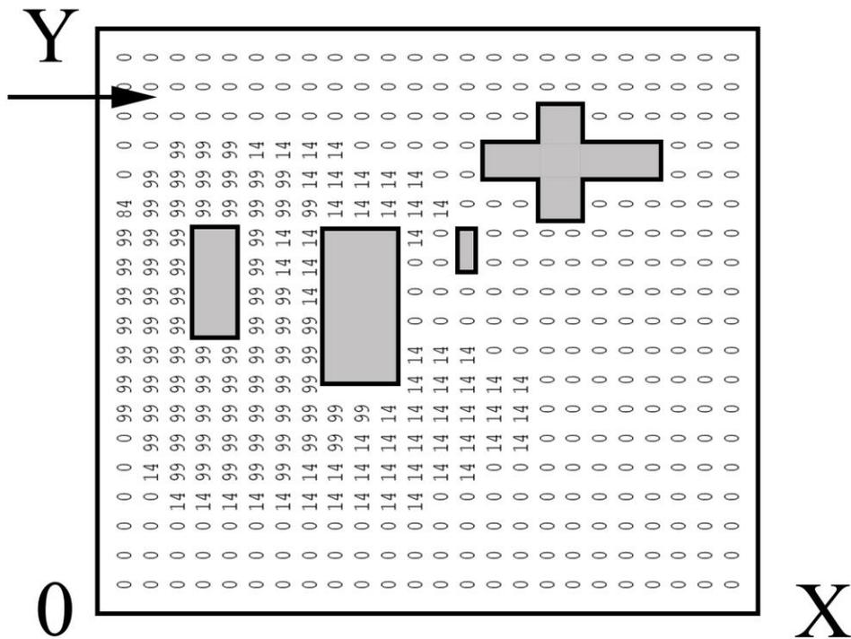
**Fig. 5.** Probability of toxic hitting,  $t= 8\text{ s}$  (for  $Cl_2$  emission)
