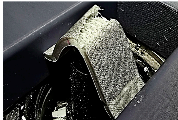
Figure 9. Elongation in the PETG gyroid-filled specimen (i.e., PETG_GyF35%).
