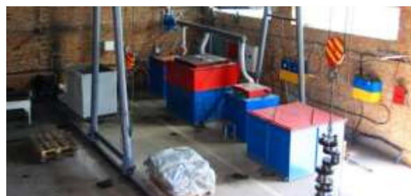
Fig. 8. Technological line of carbonitriding at “TOV KARBAZ”
