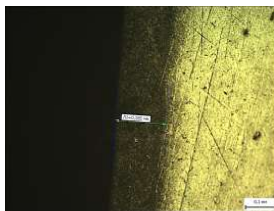
Fig. 4. Macrostructure of the cross-section of steel 4X4VMFS after carbonitriding, \times 500
