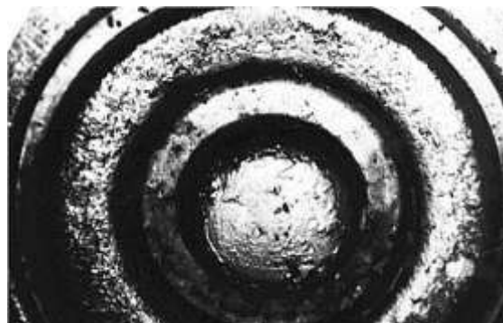
Fig. 2. Surface of tempering cracks [4]
