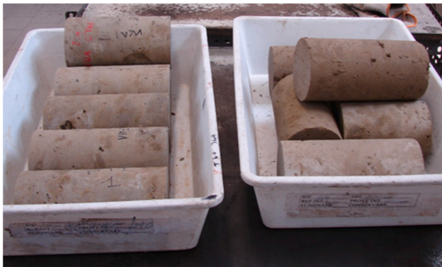
Fig. 4. Drilled core samples of grouted micropiles.
