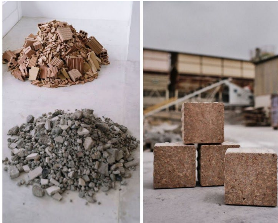
Fig. 3.20 - Brick Recycling by Crushing into Secondary Aggregate [53]
