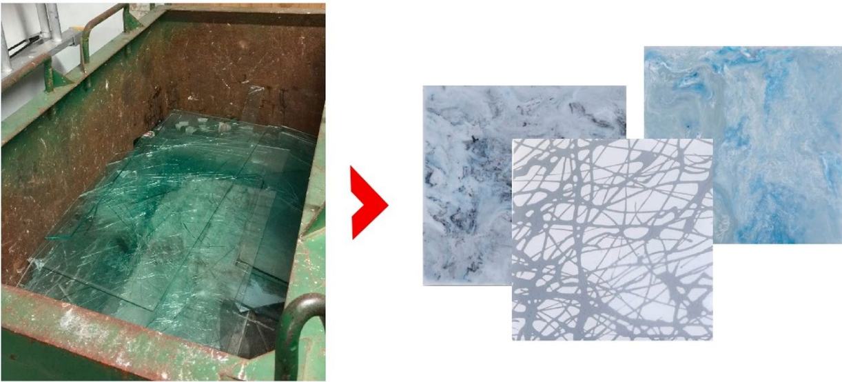
Fig. 3.21 - Recycling Window Glass for Glass Polymer Products [54]
