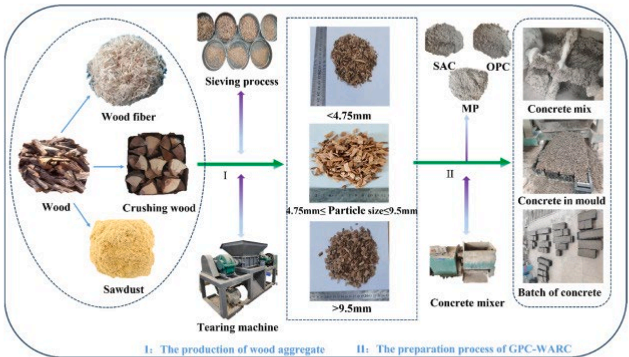
Fig. 3.1 - Production of concrete with wood aggregate [42]
