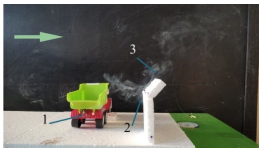
Figure 2. Experimental study of contamination zones using barrier with inclined element: 1–emission source; 2–contamination zone in front of the barrier; 3–contamination zone above the inclined element [7].
