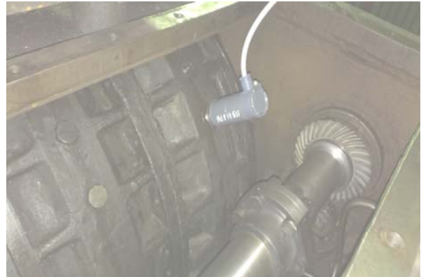
Fig. 3. Pressure sensor installation in the circulation circle of hydro apparatus
