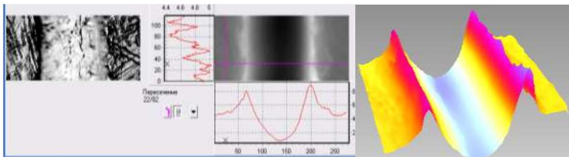
Fig. 2. Microstructure, profilograms with 2-D images and 3-D images of the friction track of the original AlSi18 (B-Sn), slowly cooled alloy
