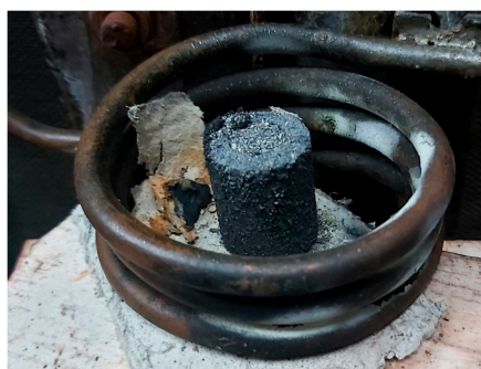
Figure 1. Melting the charge in the graphite crucible.
