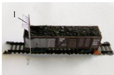
Figure 3. Model of the coal wagon with barrier: 1 – barrier (barrier + upwind wing, scenario #3).
