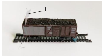
Figure.2. Model of the coal wagon with barrier: 1 – barrier (barrier + downwind wing, scenario #2).
