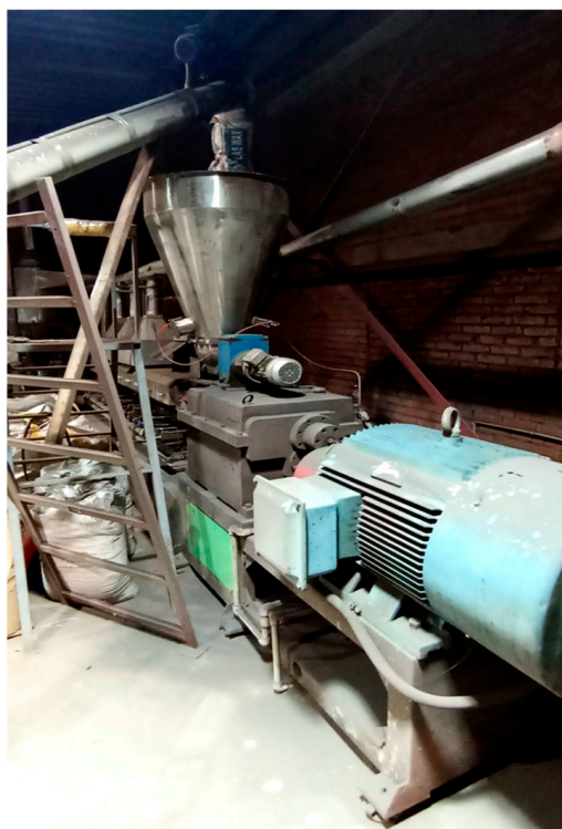
Figure 2. Twin-screw extruder SKY WIN SWMSZ-3.
