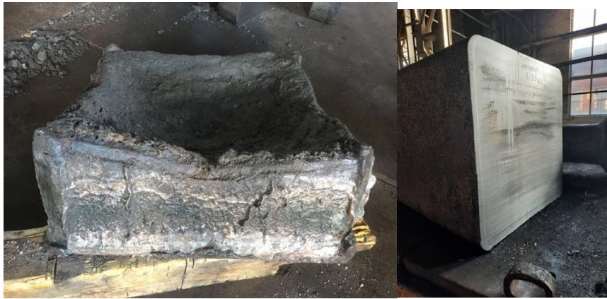
Fig. 5. Hop top cut 11% of 6,5 ton ingot 1.4541 (AISI321)
