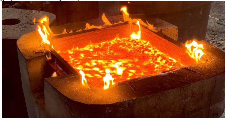
Fig. 4. Rectangular mold lined with heat-insulating boards using corner elements
