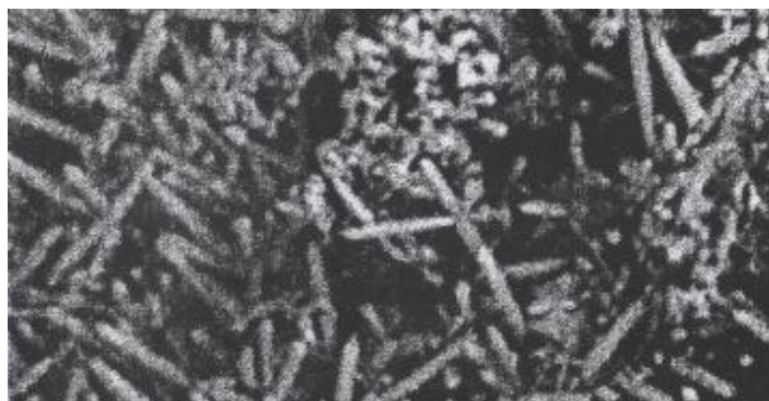
Figure 2 – Product of the TIRO process – titanium needles in a mixture with MgCl_2 granules
