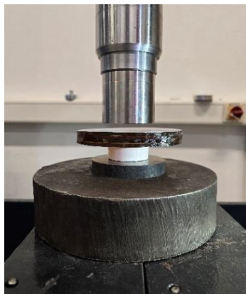
Figure 7. Measuring set-up. (One active tool (white). The metal parts are included in the machine: D80 mm, D100 mm, D250 mm, and some rubber sheets are visible above the active tool).
