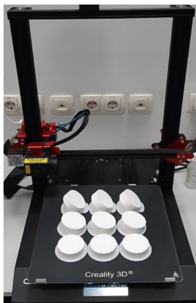
Figure 1. Illustration of printing layouts. (From the bottom up: the first row is tilted at 0^\circ , the second at 15^\circ , and the third at 45^\circ ).
