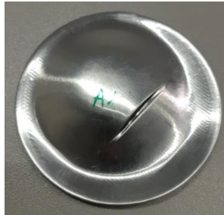
Figure 15. An example of an unsuccessful cut—0.3 mm thick Al99.5 sheets.
