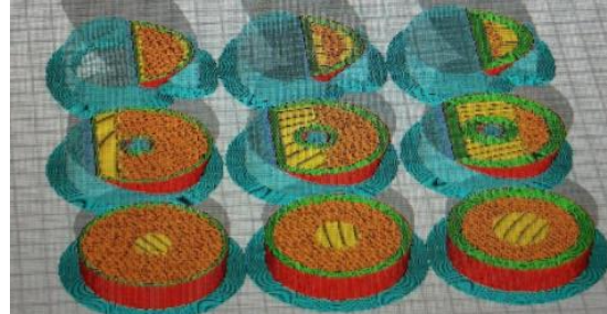
Figure 2. Tool orientation in Ultimaker Cura software. (From the bottom up: the first row is tilted at 0^\circ , the second at 15^\circ , and the third at 45^\circ ).
