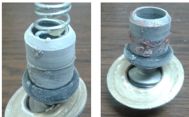
Fig. 11. View of the used Elf MULTI grease (on the left) and Vecolit EPX 00 grease (on the right) in the relay valve operating at temperature of -26^{\circ} [7]
