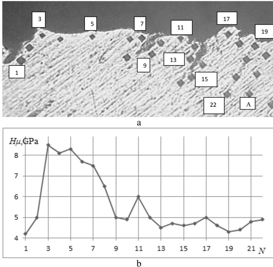
Fig. 1. The profile surface rolling of wheel's (a) and the nature of change microhardness (load on the indenter is 0,196 N) in accordance with the numbers ( $N$ ) of measurement sites (b). Magnification 350 x 1.2
