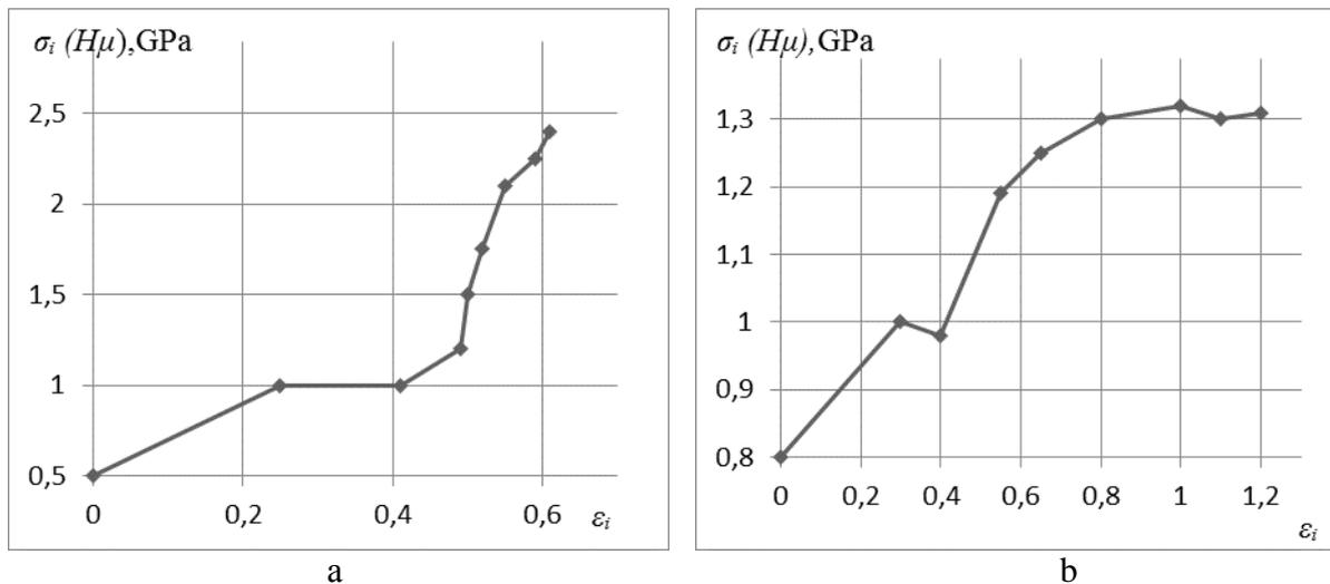
Fig. 3. The ratio of  $\sigma_i - \epsilon_i$  for volumes of metal with dispersed particles of non-metallic inclusions (a) and without them (b)
