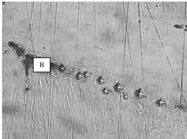
Fig. 2. The volume of metal with compactly located dispersed non-metallic inclusions after measuring microhardness. Magnification 350 x 1.6
