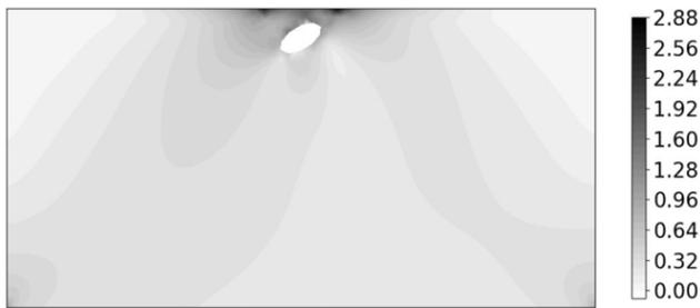
Fig. 3. Stress distribution by von Mises in the study structure within the presence of an elliptical stress concentrator,  $10^9$  Pa
