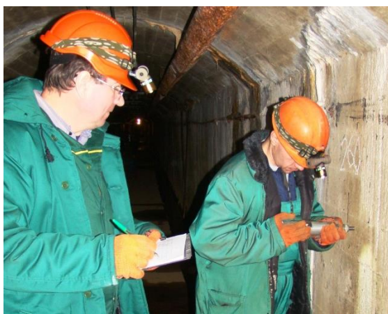
Figure 8. Strength of concrete determination with the elastic rebound method.
