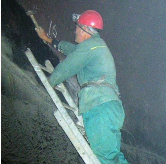
Figure 11. Excitation of vibrations in a concrete structure.
