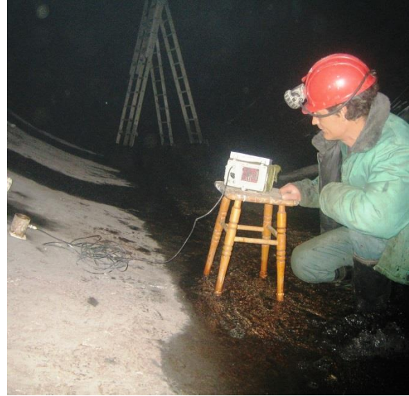
Figure 12. Distance registration of free oscillations of the structure.
