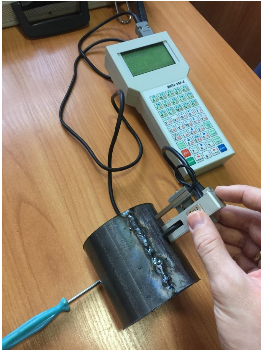
Fig. 1. General view of the TSC-1M-4 apparatus.
