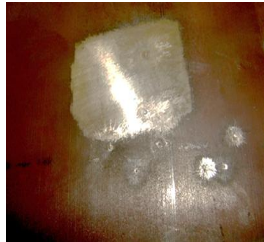
Fig. 5. Photo of a test plate for a bulletproof vest after being fired with ammunition from AK-47, AK-74 assault rifles at level 4 protection according to DSTU 8782:2018 (a);
