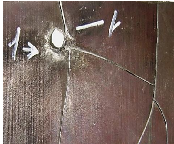
Fig. 7. Photo of a fragment from experimental plate No. 1 measuring \approx 220 \times 220 mm and 6.8 mm thick made of 38KhN3MFA steel after testing with an armor-piercing incendiary bullet 7.62x54 mm (7.62x54R) with a heat-strengthened core in a steel jacket (B32 7-B3-323) with a rifle cartridge for compliance with protection class 6 according to DSTU 8782:2018 (see clause 5.2.1, Table) for externally worn body armor (type 1)
