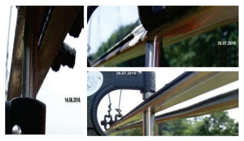
**Fig. 5.** The working surface of the contact wire at one of the control points, as of June 14, 2016
