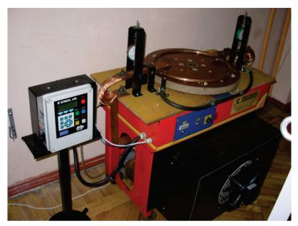
Fig. 9. Stand for testing the wear of the contact wire
