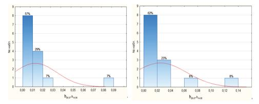
Fig. 3. The results of processing the values of the difference in heights of the left contact wire in the odd direction
