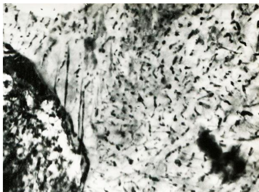
Fig. 4. Structure of low-carbon steel after isothermal transformation at a temperature of 200 °C.
