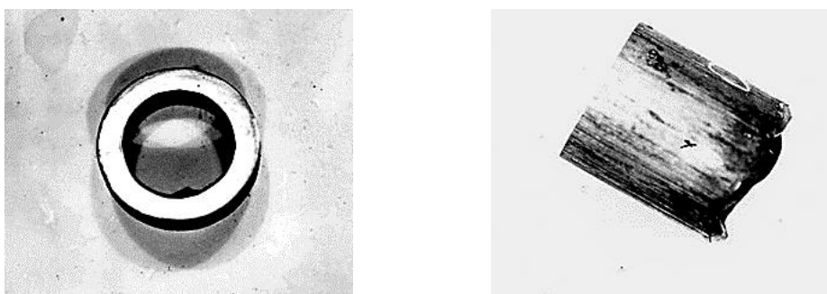
Figure 7. Macrostructure of extruded pipes and general view of templates.
