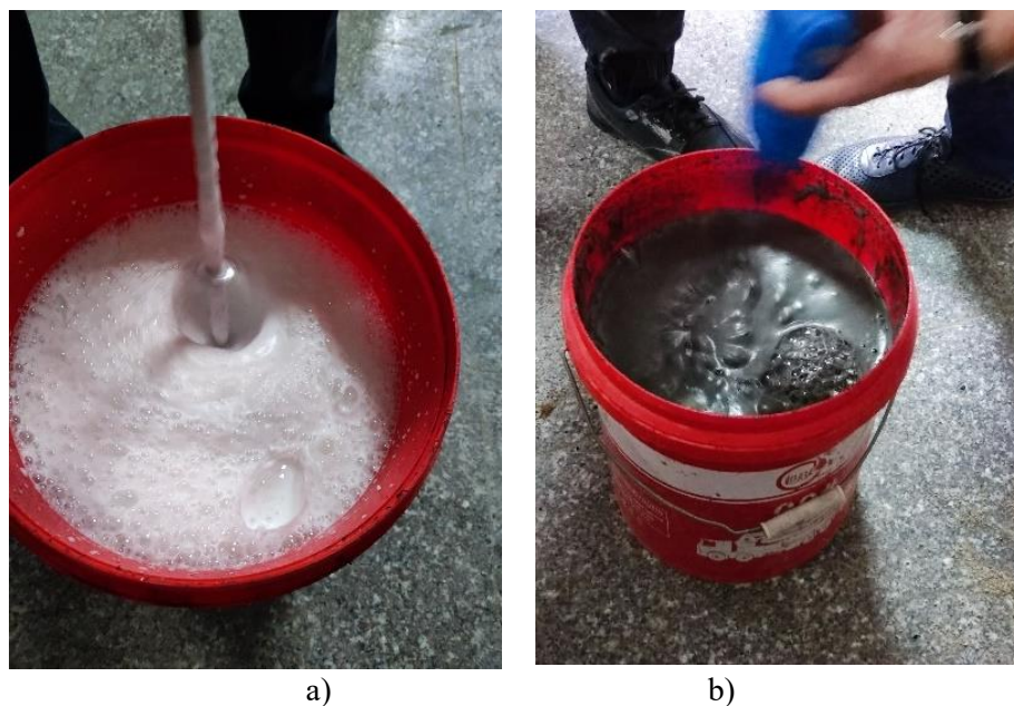
Fig. 4. Preparation a suspension of graphene oxide: a) - sodium oleate solution; b) -suspension
