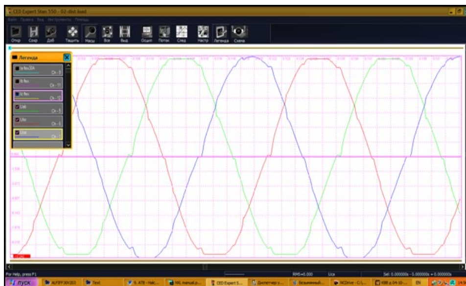
Fig. 35. Oscillograms of voltages within the considered electric motor while operating under loading
