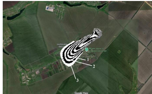
Fig. 4. Contamination zone, HCL concentration: 1 – C = 82 \text{ mg/m}^3 ; 2 – C = 61 \text{ mg/m}^3 ; 3 – C = 37 \text{ mg/m}^3
