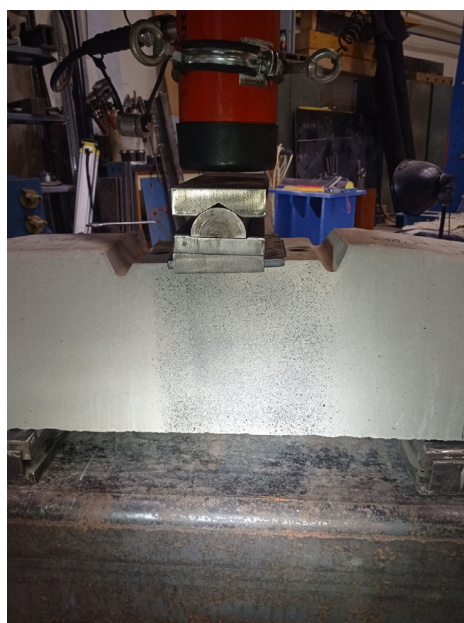
Figure 2. Pattern importance in Digital Image Correlation (DIC) measurements.
