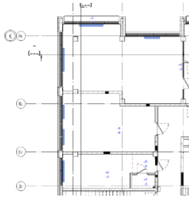
Figure 110-Placement of indoor convectors
