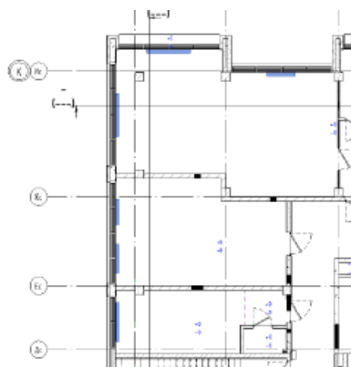
Figure 109-Automatically placed indoor radiators
