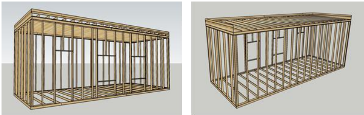
Fig. 3. 3D model of the timber carcass
