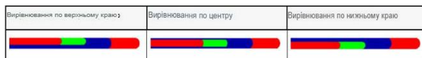
Figure 119 - table of options for aligning the base edge of pipes in relation to one to the second
