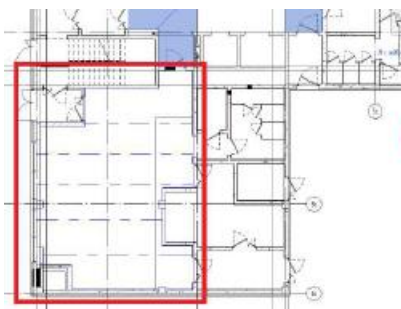
Figure 116-indication of zones for placing underfloor heating
