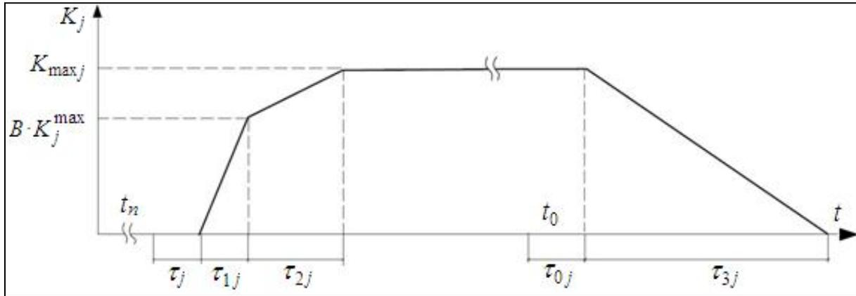
Fig. 3. Approximation of the diagram of filling and release of the brake cylinder
