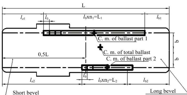
Fig. 2. Schematic of ballast arrangement
