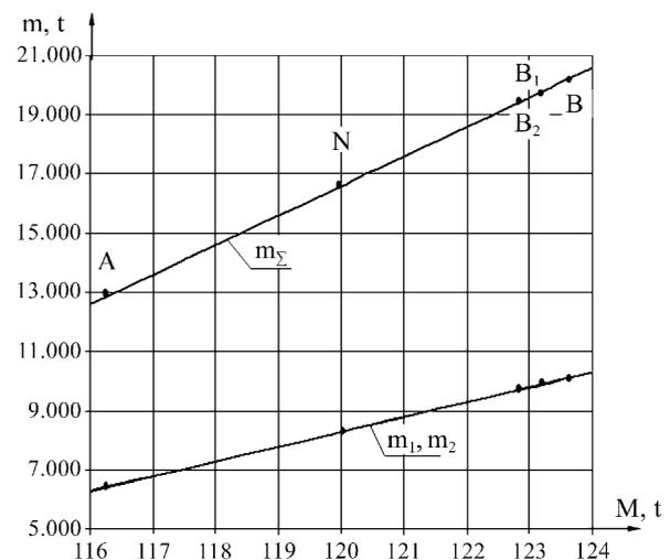
Fig. 5. Dependence of ballast mass on the mass of electric locomotive
