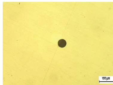
FIGURE 3: Silicate nonmetallic inclusion—Type C according to ASTM E45-18a.
