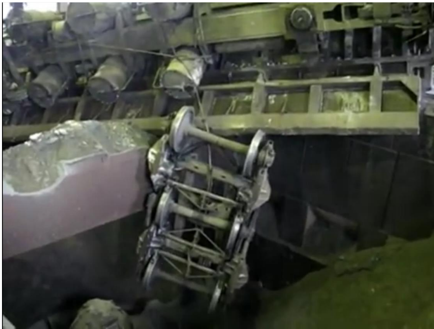
Figure 1. Overturn of a dump car during unloading of bulk material.
