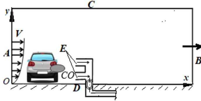
Fig. 4. Scheme of the computational domain for setting boundary conditions
