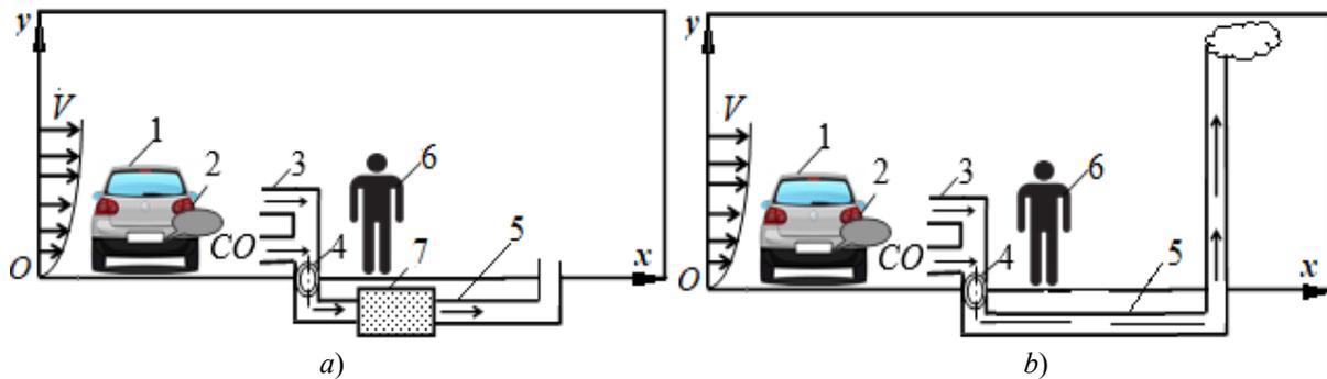
Fig. 1. Scheme of selection and removal of exhaust gases: *a* – outlet to the cleaning system; *b* – branch to a great height. 1 – motor vehicles, 2 – emission source, 3 – gas extraction pipes (nozzles), 4 – fan, 5 – gas outlet; 6 – a person in the area of the pollution source, and 7 – a cleaning system
