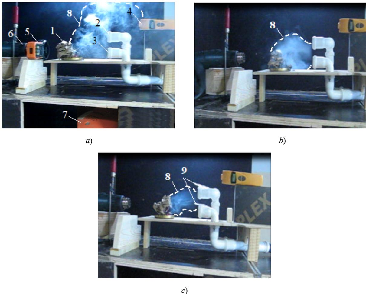
Fig. 2. Formation of the polluted zone: *a* – the exhaust fan does not work; *b* – the exhaust fan operates without guide plates  $t=14$  s; *c* – the exhaust fan operates with the same guide plates  $t=14$  s [21-22]
