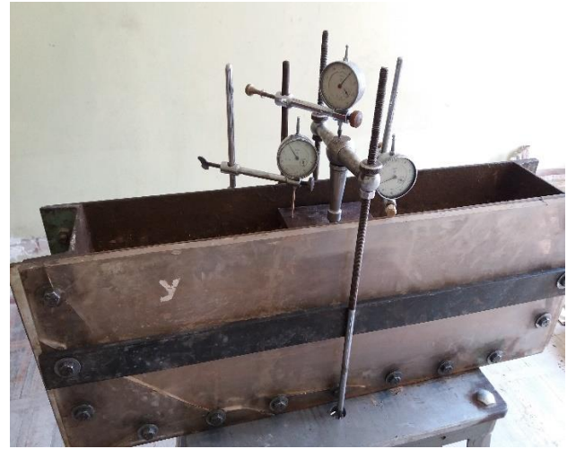
Fig. 1. Model of soil bank in trough with measuring devices.
