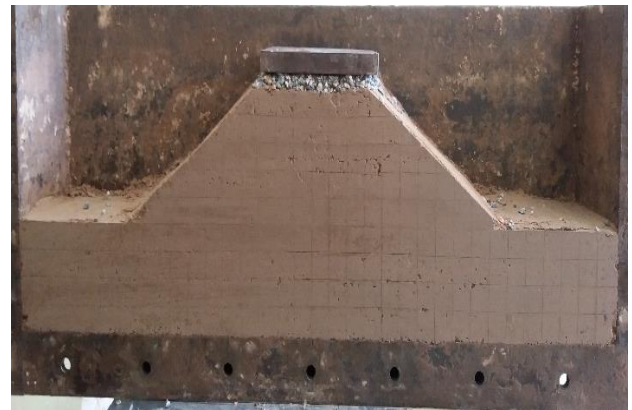
Fig. 2. Roadbed model before the test
