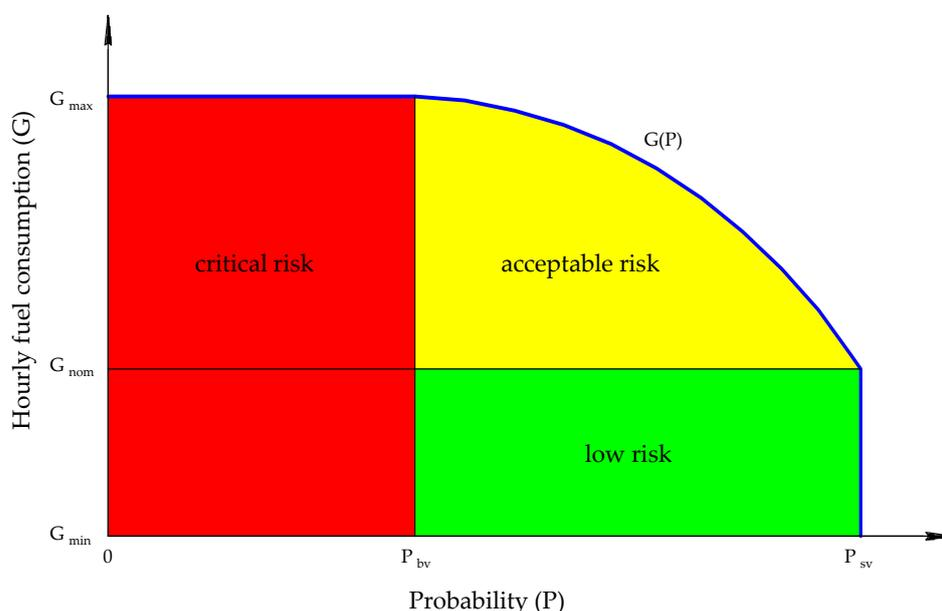
**Figure 6.** Risk zones for the dependence of hourly fuel consumption on the probability of the failure-free operation of LDEs.
