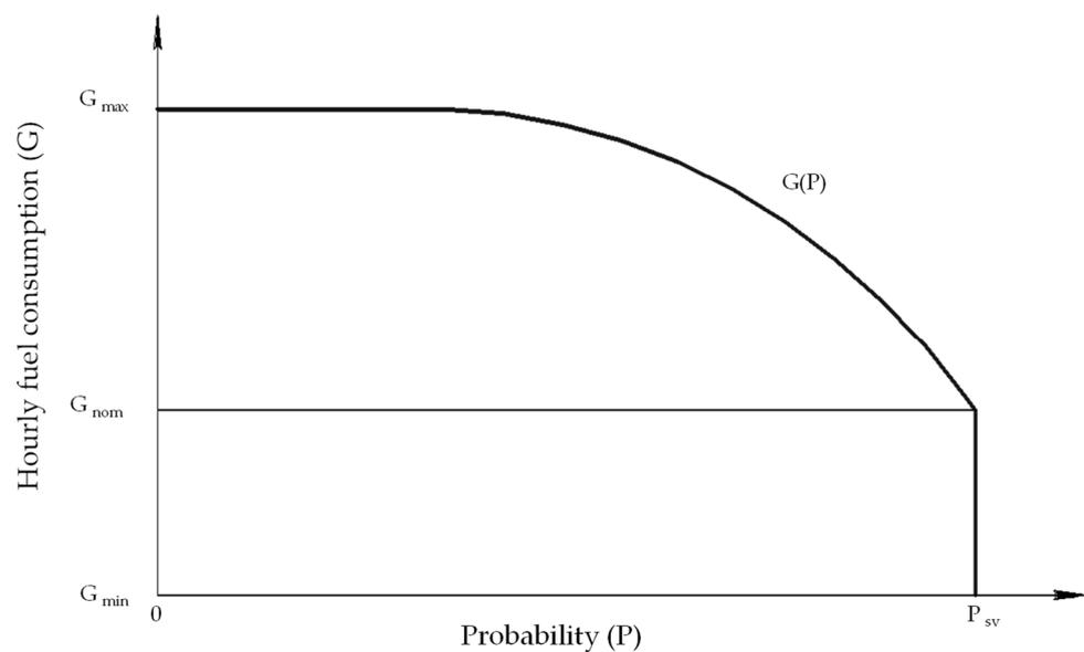
**Figure 5.** Dependence of hourly fuel consumption on the probability of the failure-free operation of LDEs.
