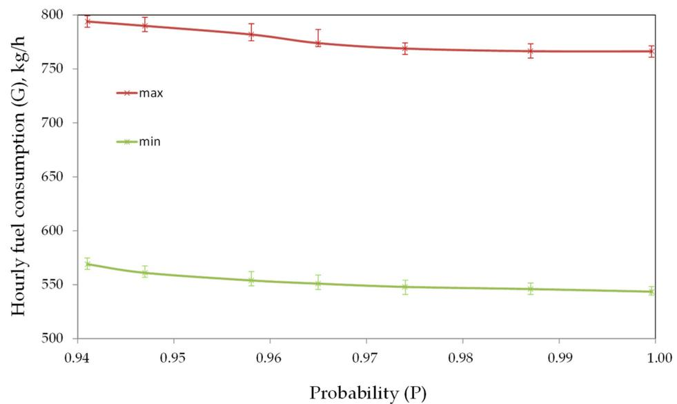
**Figure 4.** Experimental dependence of hourly fuel consumption of 5D49 diesel engines on the probability of failure-free operation.
