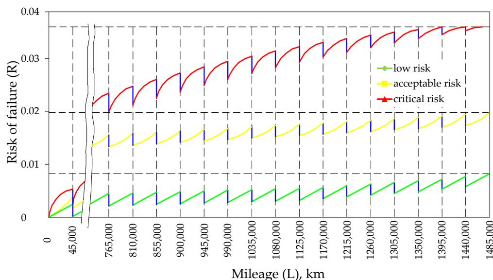
**Figure 10.** Theoretical maintenance system and the risk of failures of 5D49 diesel engines depending on the mileage.
