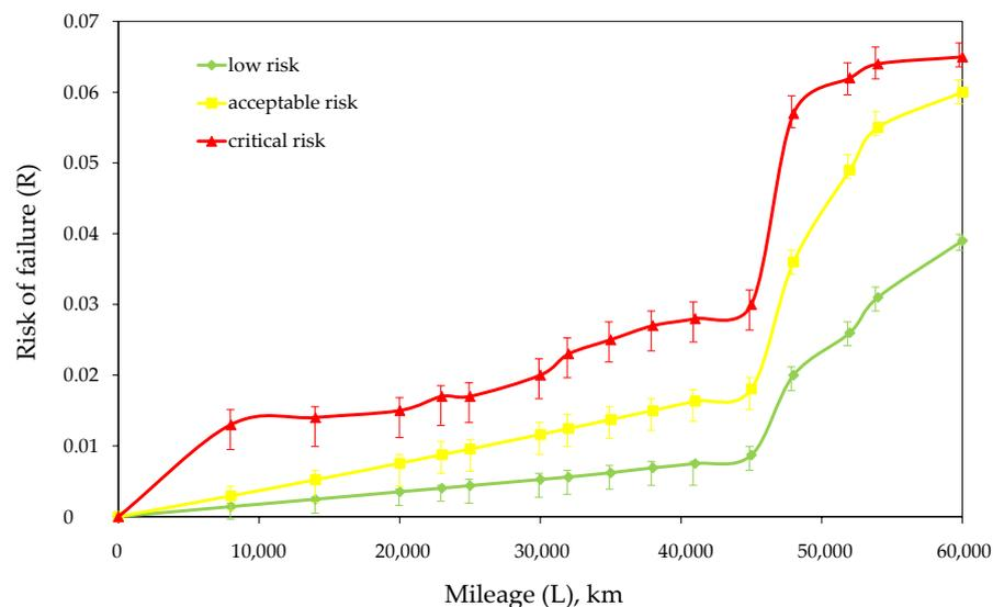
**Figure 9.** Experimental results of the risk of failures of 5D49 diesel engines in a locomotive depot on the mileage.
