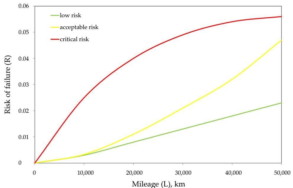
**Figure 7.** Dependence of the risk of failures of 5D49 diesel engines on the mileage by hourly fuel consumption.
