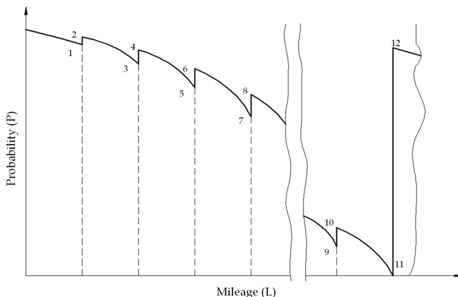
**Figure 3.** Probability of a failure-free operation of an LDE depending on the mileage during maintenance and repair operations.
