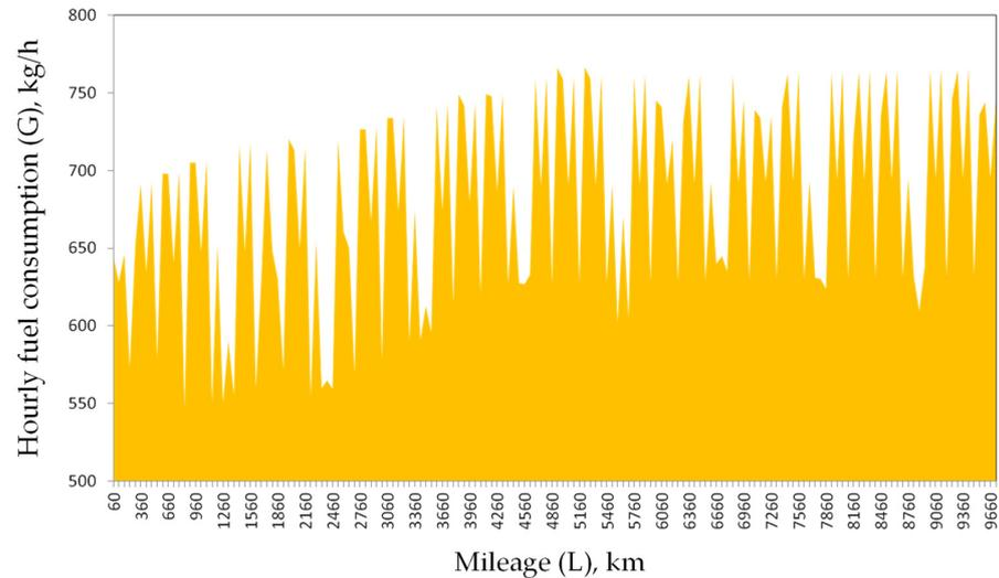
**Figure 8.** Hourly fuel consumption of 5D49 diesel engines depending on the mileage of a locomotive.
