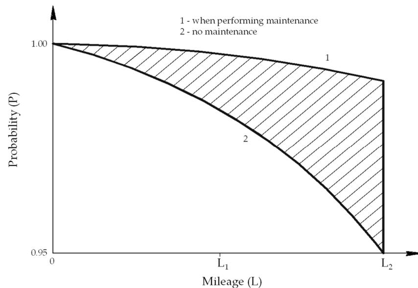
**Figure 2.** Probability of a failure-free operation of an LDE during operation, depending on the mileage [1,6].
