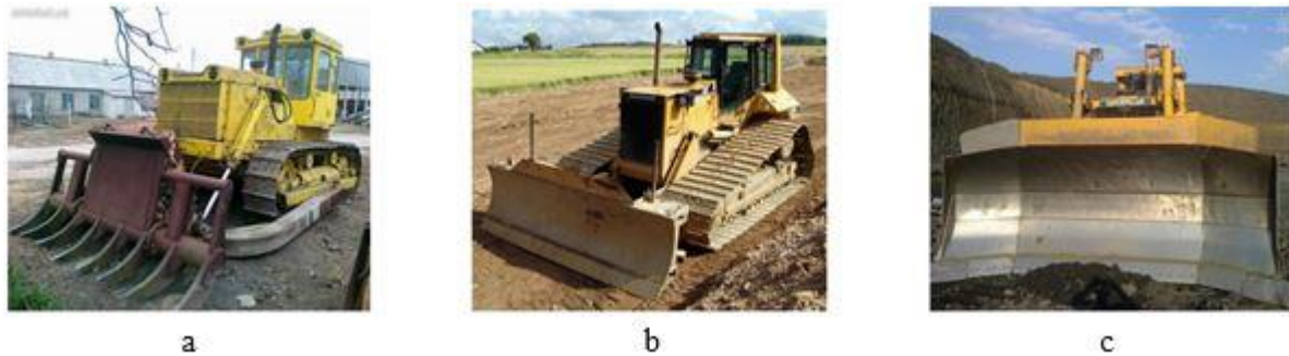
Figure 5. Similar bulldozers for the development of a new type spatial knife system: a – a snubber; b – with a rotary blade; c – with a non-return blade.
