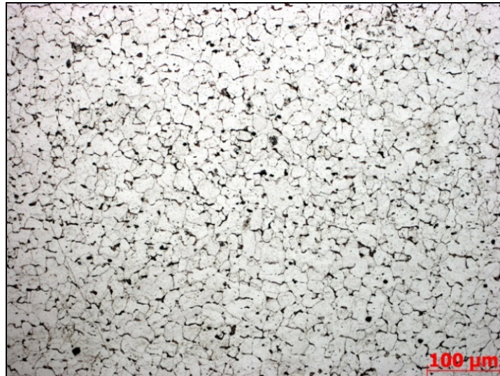
Fig. 1 - The structure of a hot-rolled billet for the manufacture of welded pipes, steel grade 3PS
