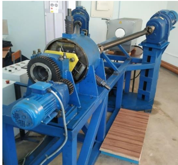
Figure 1 – Radial-shear rolling mill SVP-08
